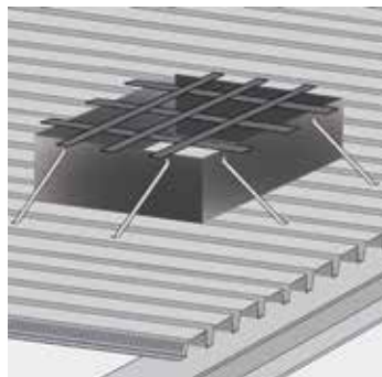
8 ■ Install fall protection for openings and block-outs
