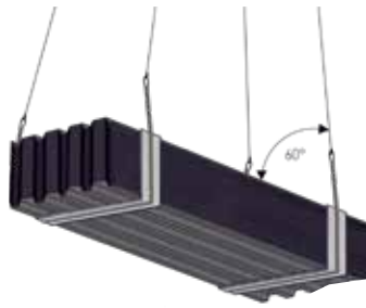
2 ■ Use adequate slings and lifting tools to unload bundles
