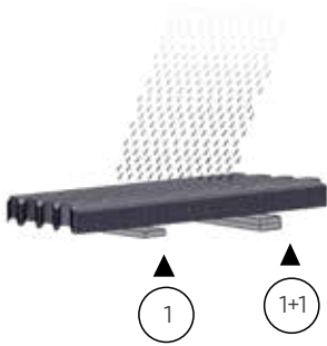
10 ■ Store profile bundles with a slight slope to avoid accumulation of rainwater
