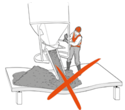
19 ■ Avoid any concrete accumulation while concreting
