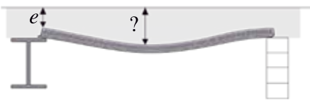
7 ■ Survey concrete thicknesses using a pin rather than a laser level which is not considering deflection of the main structures
