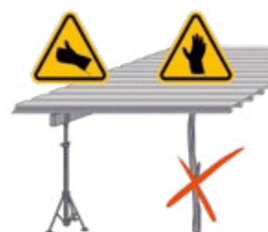
9 ■ Use a suitable prop equipment
