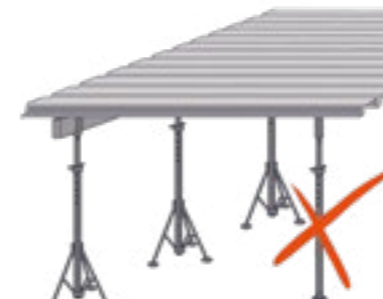
17 ■ In case of propping, use a classical formwork beams instead of single props
