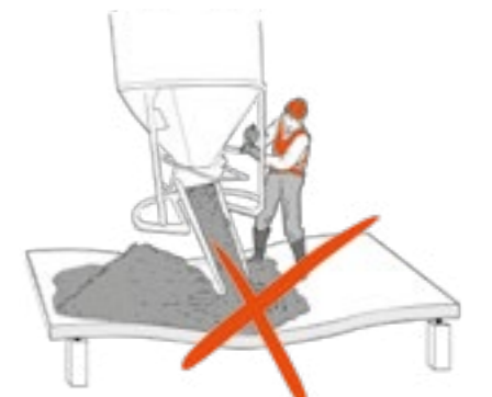
19 ■ Avoid any concrete accumulation while concreting
